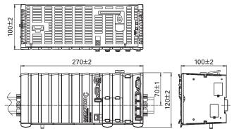
Fig. 2: External dimensions of the new model
